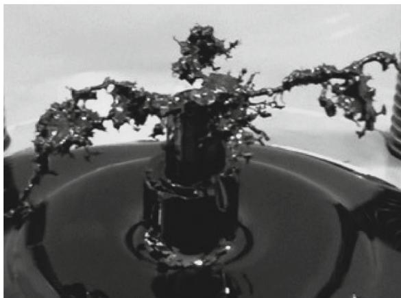
Fig. 3. Tree-like structure at the end of the electrode formed in a discharge in the hydroconversion product.
