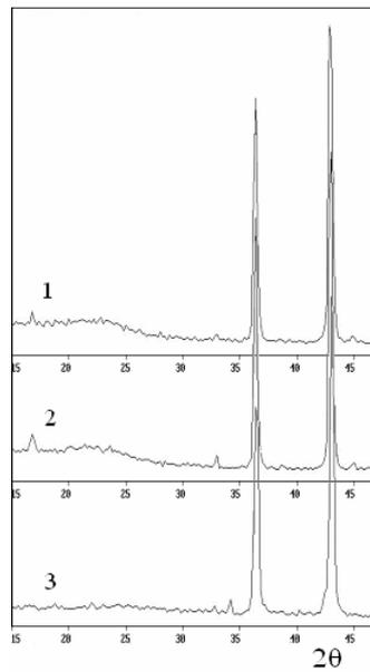
**Figure 2:** XRD patterns for  $ZnAl_2O_4:Eu$  samples synthesized in SCW-Am as a function of the doping concentration in reaction medium: (1) 0.8; (2) 1.2; (3) 1.6 mol%.
