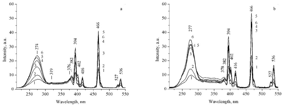
**Figure 6:** Excitation spectra of Eu (0.4 and 4 mol%)-doped gahnite samples synthesized: (a) in SCW-Am, (b) in SCW. (Emission 612 nm). Content of europium, mol%: (1) 0.4, (2) 0.8, (3) 1.2, (4) 1.6, (5) 2, (6) 4.
