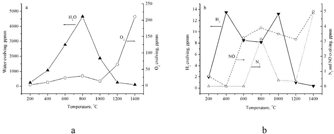
**Figure 9:** Gases evolving at stepwise vacuum heating of Eu (0.4 mol%)-doped gahnite samples synthesized in SCW-Am.: H<sub>2</sub>O and O<sub>2</sub> – a, H<sub>2</sub>, N<sub>2</sub>, NO – b.
