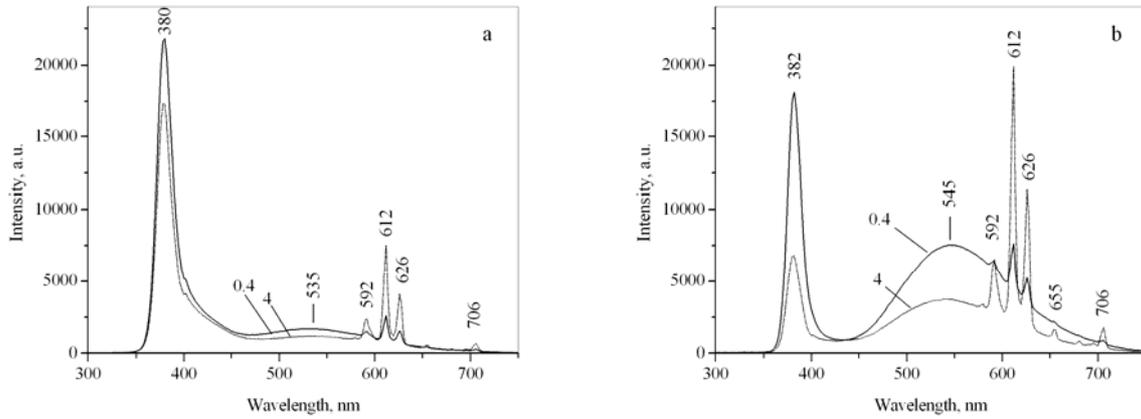
**Figure 5:** Emission spectra of Eu (0.4 and 4 mol%)-doped gahnite samples synthesized: (a) in SCW-Am, (b) in SCW. (Excitation 254 nm).
