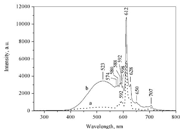
**Figure 8.** Emission spectra after annealing in air at 1200 C for 1 h of Eu (4 mol%)-doped gahnite samples synthesized: (a) in SCW-Am, (b) in SCW. (Excitation 254 nm).
