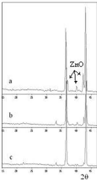
**Figure 1:** XRD patterns for Eu (1.2 mol%)-doped  $ZnAl_2O_4$  samples synthesized in SCW: (a) as prepared, (b) after annealing at 1000 C, (c) at 1200 C.
