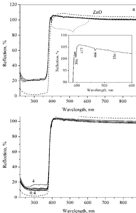
**Figure 4:** DR spectra initial zinc oxide (dotted line) and samples of Eu (0.4-4 mol%)-doped gahnite synthesized in: (a) SCW-Am., (b) SCW.
