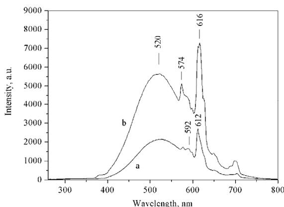
**Figure 7.** Emission spectra after annealing in air at 1200 C for 1 h of Eu (0.4 mol%)-doped gahnite samples synthesized: (a) in SCW-Am, (b) in SCW. (Excitation 254 nm).
