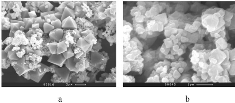
**Figure 3:** SEM micrographs of Eu (1.6 mol%)-doped gahnite samples synthesized: (a) in SCW, (b) in SCW-Am.
