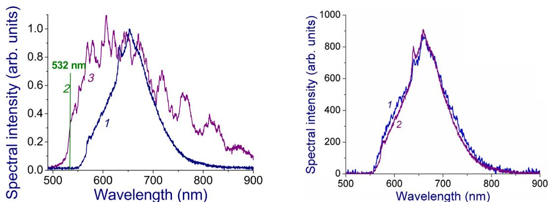
FIG. 5. (a) Spectra of NV center emission from a nanodiamond-doped hollow-core PCF (1), 532-nm excitation radiation (2), and fiber transmission (3). (b) Spectra of NV center emission from nanodiamond-doped hollow-core PCF (1) and from a glass substrate (2). The density of NV centers is  $10^4$  per 1 cm of fiber.
