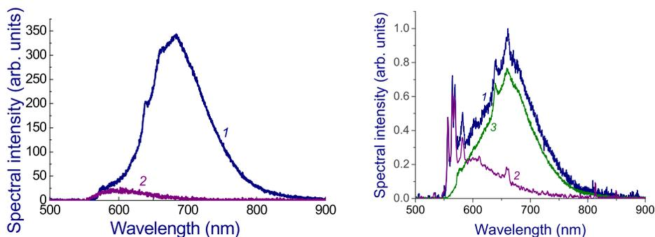
FIG. 4. Spectra of NV center emission from a nanodiamond-doped ultrasmall-core PCF (1), the Raman background from the same fiber (2), and NV center emission from a glass substrate (3). The density of NV centers is  $5 \times 10^4$  (a) and  $10^3$  (b) per 1 cm of fiber.
