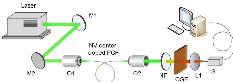
FIG. 3. Diagram of the experimental setup: M1, M2, mirrors; O1, O2, objectives; NF, notch filter; CGF, color-glass filter; L1, lens; S, spectrometer.
