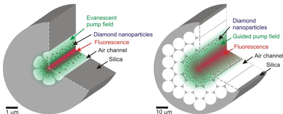
FIG. 2. Coupling nitrogen vacancies to waveguide modes of a nanodiamond-doped solid-core (a) and hollow-core (b) photonic crystal fiber.
