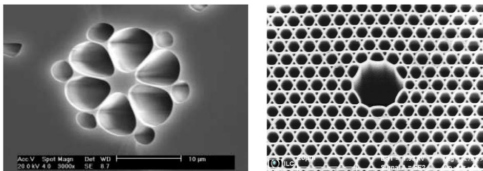
FIG. 1. SEM images of photonic-crystal fibers: (a) an ultrasmall-core PCF, (b) hollow-core PCF.
