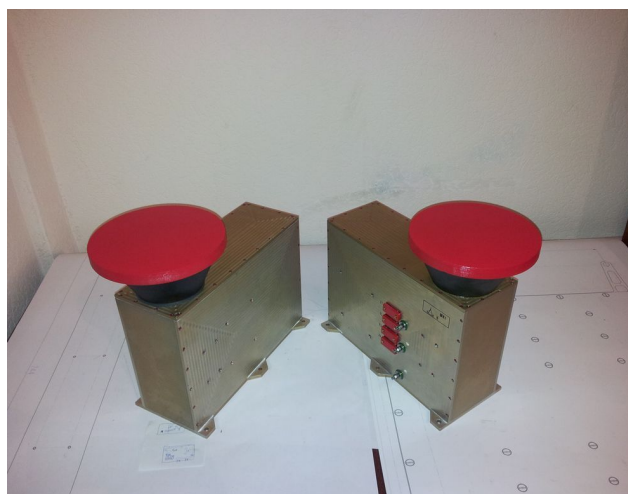
Figure 2. Wide field optical camera units from Lomonosov satellite scientific payload.
