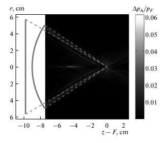
**Fig. 7.** Magnitude of a difference between the absolute values of the pressure amplitude in the solutions to the full diffraction and the parabolic models normalized to the pressure amplitude at the focus  $\Delta p_{\rm A}/p_F$ , in the plane passing through the beam axis. Here, r is the radial coordinate, and z - F is the axial coordinate with the origin at the focus. The two-dimensional distribution also depicts the spherical and equivalent sources.
