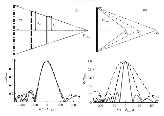
**Fig. 2.** Pressure amplitude distributions on the beam axis normalized to the corresponding maximum values,  $p_{\rm A}/p_{\rm max}$ , calculated by the parabolic approximation for sources with identical (a) and different (b) F-numbers  $\alpha = F/2a$ . Examples are given for transducers of 1.5 MHz frequency and (a)  $F_{1,2,3} = 16$ , 12, and 8 cm,  $\alpha = 1.5$ ; (b)  $F_{1,2,3} = 8$ , 12, and 16 cm,  $\alpha = 1$ , 1.5, and 2.
