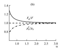
Fig. 5. Scaling curves for F-number (a), focal distance, and initial pressure amplitude (b) for the equivalent source in the parabolic model as functions of the parameters of the spherical transducer.
