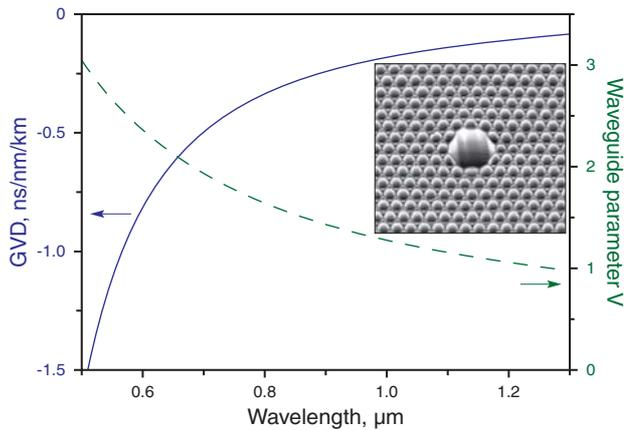
**Figure 1** (online color at [www.lphys.org](http://www.lphys.org)) The group-velocity dispersion (GVD, solid line) and waveguide parameter  $V$  (dashed line) calculated as a function of the radiation wavelength for a benzene-filled PCF structure shown in the inset. The fiber core diameter is  $4 \mu\text{m}$
