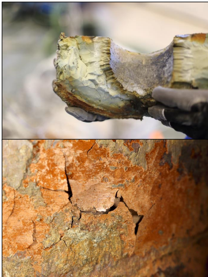
Fig. 1. Left: In several bentonite blocks centrosymmetrical white precipitates and significant corrosion at the iron heater interface could be seen. Right: At some locations on the heater a thin layer was found loosely bound to the heater associated with corrosion products and clay minerals.
