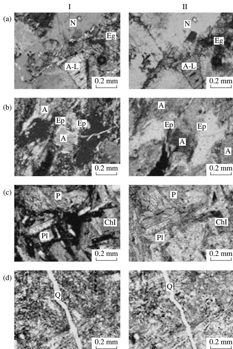
**Fig. 1.** Photos of thin sections (I—crossed nicols, II—parallel nicols): (a) nepheline syenite, (b) amphibolite, (c) relicts of the ophitic (diabase) structure in the metamorphized gabbro diabase, (d) quartz-filled veins in the metamorphized gabbro diabase. Designations: (N) nepheline, (Eg) aegirine, (A-L) minerals of the astrophyllite-lamprophyllite group, (A) amphibole, (Ep) epidote, (P) pyroxene, (Pl) plagioclase, (Chl) chlorite, and (Q) quartz.
