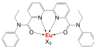
Figure 1. Structure of studied europium complexes with ligand based on 2,2'-bipyridyldicarboxylic acid (counterion X = \text{CF}_3\text{CO}_2 (1), \text{NO}_3 (2), \text{Cl} (3)).
