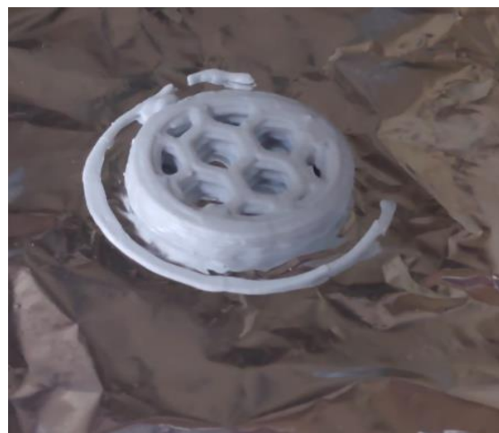
Figure 2. Sample after extrusion 3D-printing prepared from highly concentrated hardening suspensions ( \text{Ca}(\text{PO}_3)_2/\text{Ca}_2\text{P}_2\text{O}_7 = 0/100 ).
