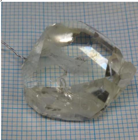
154 **Figure 2.** The Yb:YMgB<sub>5</sub>O<sub>10</sub> single crystal grown in 20wt.% Yb:YMBO - 80wt.% K<sub>2</sub>Mo<sub>3</sub>O<sub>10</sub> system (1
