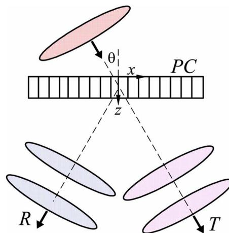
FIG. 1. (Color online) Schematic diagram of doubling of the number of laser pulses caused by splitting of an incident pulse within PC at the Bragg diffraction in the Laue geometry;  $T$  and  $R$  are transmitted and diffractively reflected pairs of pulses at the PC output.
