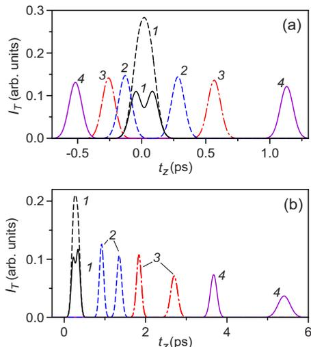
FIG. 6. (Color online) Dynamics of the transmitted pulse intensity  $I_T(z, t_z)$  at PC thicknesses  $z=(1)$  0.05, (2) 0.2, (3) 0.4, and (4) 0.8 mm. The parameters of the incident pulse and PC are as follows:  $\tau_0=0.1$  ps,  $\lambda_0=0.8$   $\mu\text{m}$ ,  $\xi=0.5$ ,  $n_1=1.5$ , and  $\delta_0=0.1$ ; the period  $d=(a)$  3 and (b) 0.8  $\mu\text{m}$ . The dashed curves 1 are related to the diffracted pulse at  $z=0.05$  mm.
