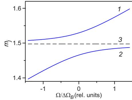
FIG. 4. (Color online) Frequency dependences of the effective refractive indices (1)  $m_1$ , (2)  $m_2$ , and (3)  $\text{Re}(\gamma_0)$  for a PC with the period  $d = 1$   $\mu\text{m}$ ,  $\xi = 0.5$ ,  $n_1 = 1.5$ , and  $\delta_0 = 0.1$ ; the wavelength  $\lambda_0 = 0.8$   $\mu\text{m}$ .
