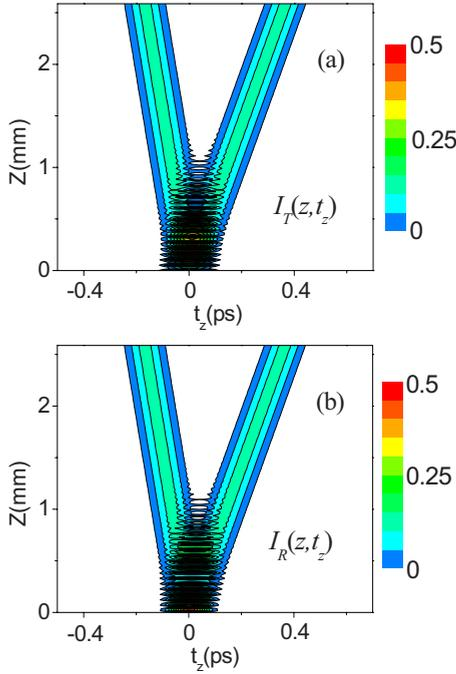
FIG. 2. (Color online) Spatial-temporal dynamics of the incident pulse evolution inside a PC, one pulse splits on two pulses. Intensities of (a) transmitted  $I_T(z, t_z) = |E_0(z, t_z)|^2$  and (b) diffracted  $I_R(z, t_z) = |E_h(z, t_z)|^2$  waves calculated by expression (17) (arb. units). The parameters of the incident pulse and PC are as follows:  $\tau_0 = 0.1$  ps,  $\lambda_0 = 0.8$   $\mu\text{m}$ ,  $\xi = 0.5$ ,  $n_1 = 1.5$ ,  $\delta_0 = 0.1$ , and  $d = 3$   $\mu\text{m}$ .
