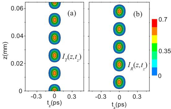
FIG. 3. (Color online) Initial stage of pulse evolution represented in Fig. 2. The superposition of four waves  $E_{01,2}$  and  $E_{h1,2}$  leads to so-called pendular solution when energy is periodically completely transferred from (a) the transmitted  $I_T(z, t_z)$  to (b) the diffracted  $I_R(z, t_z)$  waves and vice versa (arb. units).
