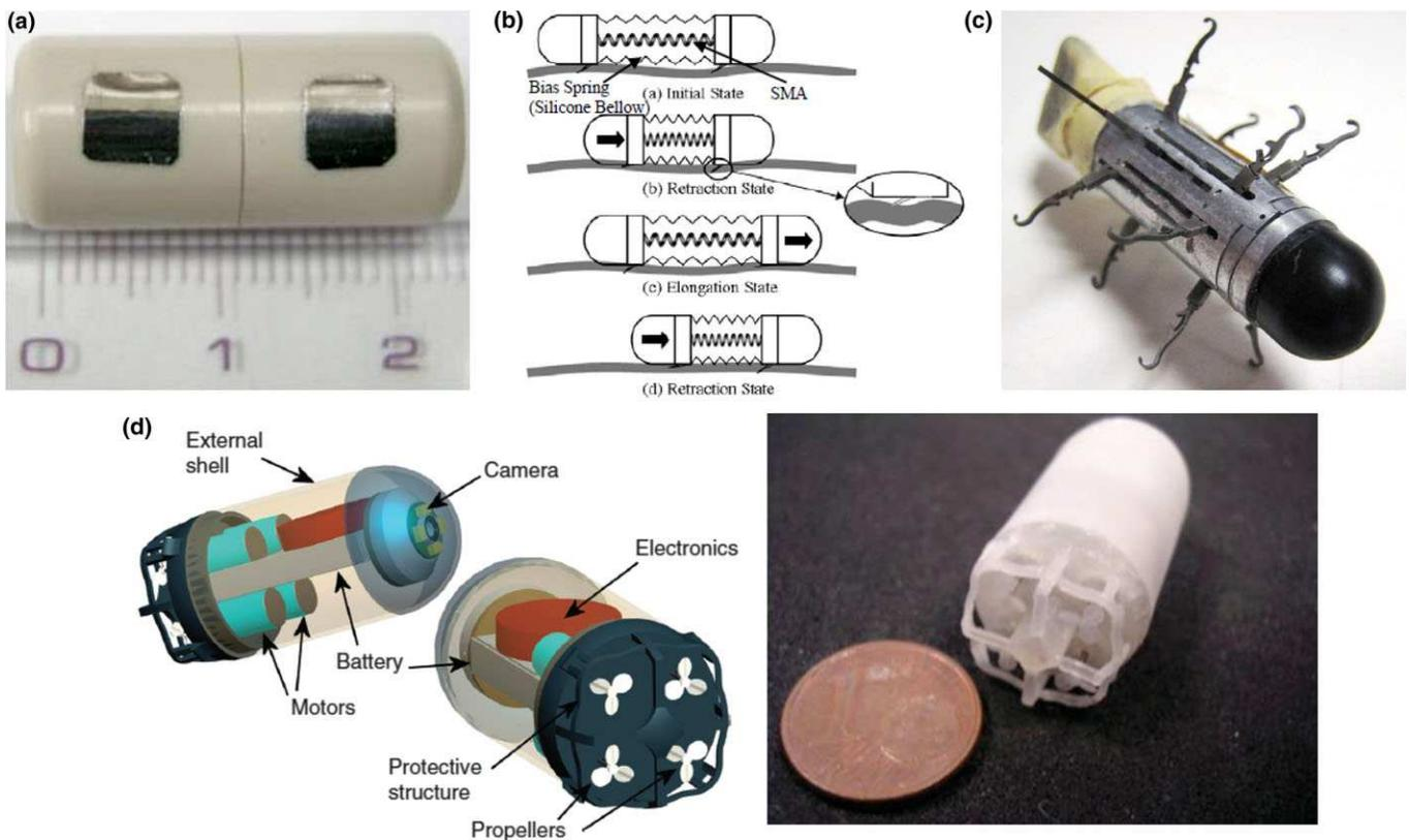
FIG. 2. Advanced WCE prototypes: (a) Capsule with patch electrodes for intestinal locomotion via electrically induced muscular contraction.<sup>33</sup> (b) SMA-based “Earthworm” capsule for intestinal locomotion.<sup>37</sup> (c) Twelve-legged capsule for crawling motion in the intestine.<sup>38</sup> (d) capsule with four propellers for swimming in a liquid-distended stomach.<sup>40</sup> [Color figure can be viewed at [wileyonlinelibrary.com](http://wileyonlinelibrary.com)]
