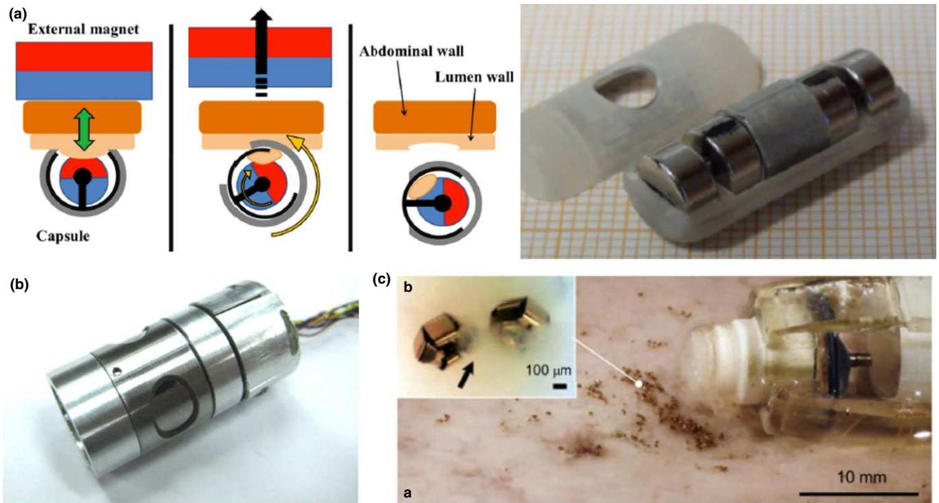
FIG. 7. Biopsy sampling capsules: (a) Mechanism of tissue retrieval developed by Simi et al.,<sup>181</sup> (b) Capsule with rotary blades released using shape memory alloys by Kong et al.,<sup>182</sup> (c) Deployment of magnetic microgrippers for biopsy sampling by Yim et al.<sup>183</sup> [Color figure can be viewed at [wileyonlinelibrary.com](http://wileyonlinelibrary.com)]
