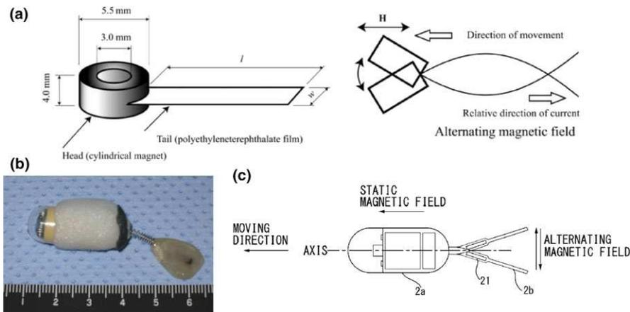
FIG. 5. (a) Magnetic swimming mechanism by use of alternating magnetic fields and a flexible tail by Sudo *et al.*<sup>128</sup> (b) Capsule with permanent magnet in a fin by Morita *et al.*<sup>132</sup> (c) Schematic from patent filing showing fish-like robot.<sup>135</sup> [Color figure can be viewed at [wileyonlinelibrary.com](http://wileyonlinelibrary.com)]
