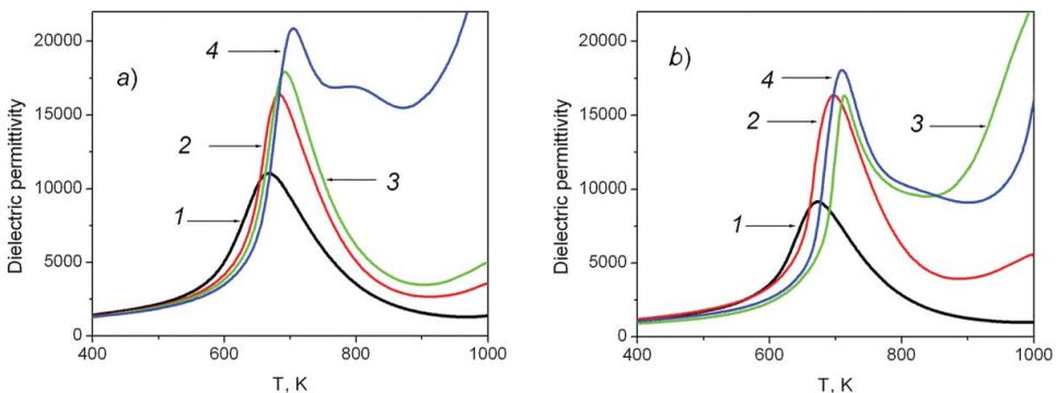
**Figure 3.** Temperature dependencies of dielectric permittivity of ceramics BSPT1 (a) and BSPT2 (b) modified by KCl/LiF additives (on cooling). Initial samples – curves 1, samples with 5 w. % of KCl/LiF – curves 2, with 10 w. % – curves 3, with 15 w. % - curves 4. Measuring frequency  $f = 1 \text{ kHz}$ .
