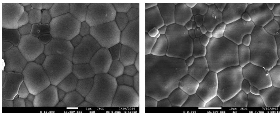
**Figure 2.** The microstructure of the BSPT1 ceramics modified by 5 w. % (left) and 15 w. % (right) of the KCl/LiF additives. Scale bars –  $1 \mu\text{m}$  (left) and  $10 \mu\text{m}$  (right).
