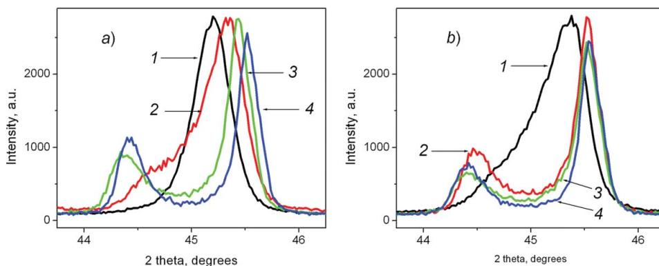
**Figure 1.** Parts of the X-ray diffraction patterns of the BSPT1 (a) and BSPT2 (b) ceramics: initial samples – curves 1, samples modified by the KCl/LiF additives in amounts of 5 w. % - curves 2, 10 w. % - curves 3, and 15 w. % - curves 4.
