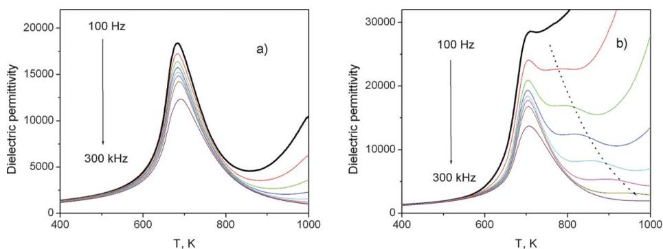
**Figure 4.** Temperature dependencies of dielectric permittivity of ceramics BSPT1 modified by 5 w. % KCl/LiF (a) and 15 w. % KCl/LiF (b) (on cooling). Measuring frequencies  $f = 100, 300$  Hz, 1, 3, 10, 30, 100, 300  $\mu$ Hz.
