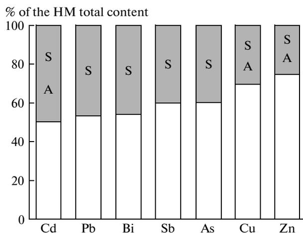
**Fig. 2.** Accumulation of the HMs in the surface layers of soils in the EAO of Moscow as a result of increased capacity (gray color) of the geochemical barriers: S is a sorption barrier, A is an alkaline barrier.
