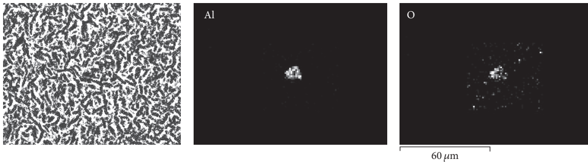
FIGURE 4: SE image and EDS maps of aluminum and oxygen distribution for the left breakdown site in Figure 2(b).
