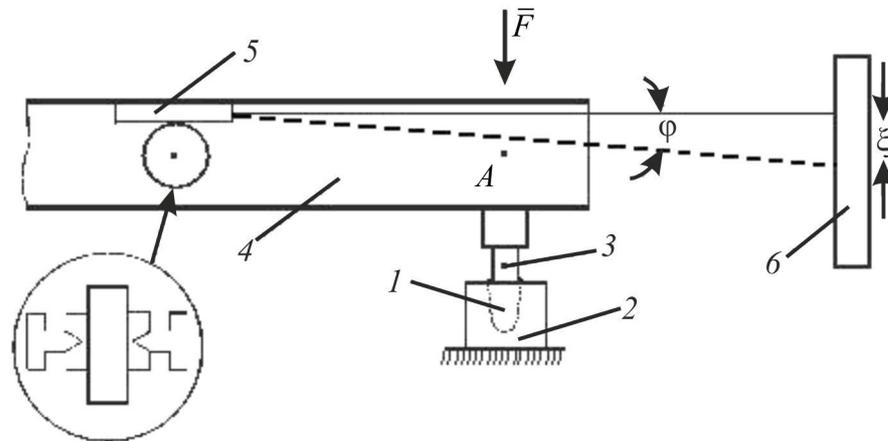
Fig. 2. Scheme to determine the stiffness coefficients corresponding to the translational degrees of freedom: 1 – implant; 2 – analogue bone; 3 – pin; 4 – lever-rocker; 5 – laser; 6 – screen
