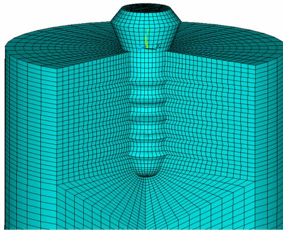
Fig. 5. Implant  $h = 13$  mm screwed into a cylindrical sample of material boxil. Fourth part is cut specifically (ordered grid), the sample is  $D = 20$  mm,  $H = 30$  mm
