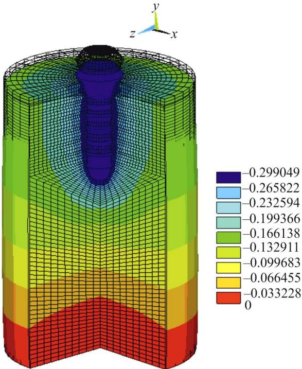
Fig. 6. Displacement along y-axis: implant  $h = 13$  mm,  $d = 4$  mm, the vertical force  $F = 5$  N, the boundary condition: the bottom of sample is fixed,  $\Delta Y_{\max} = 0.299$  mm
