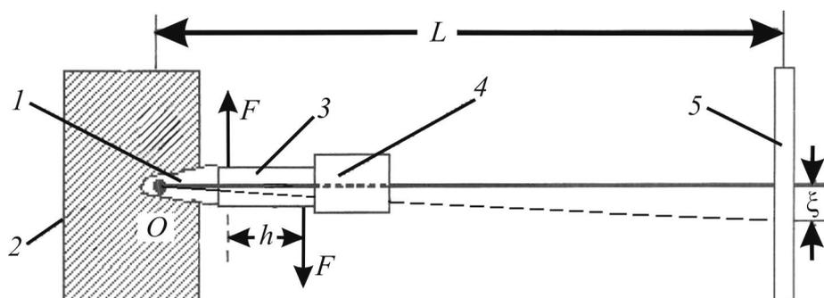
Fig. 9. Scheme for the implant turning angles measuring
