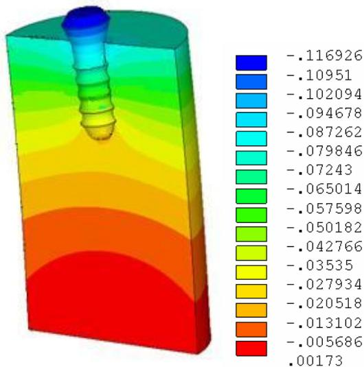
Fig. 12. Displacement along axis *X* (horizontal): implant  $h = 13$  mm,  $d = 4$  mm, fixed bottom of the sample. The maximum value of the implant displacement along *X*-axis is equal to 0.1169 mm
