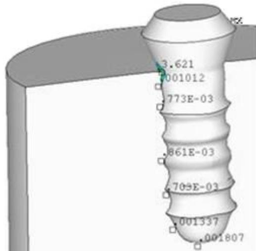
Fig. 13. The von Mises stress distribution: implant  $h = 13$  mm,  $d = 4$  mm, the bottom of the sample is fixed;  $\sigma_{\max} = 0.01807$  MPa =  $0.001807$  kg/mm<sup>2</sup> at the base of the implant
