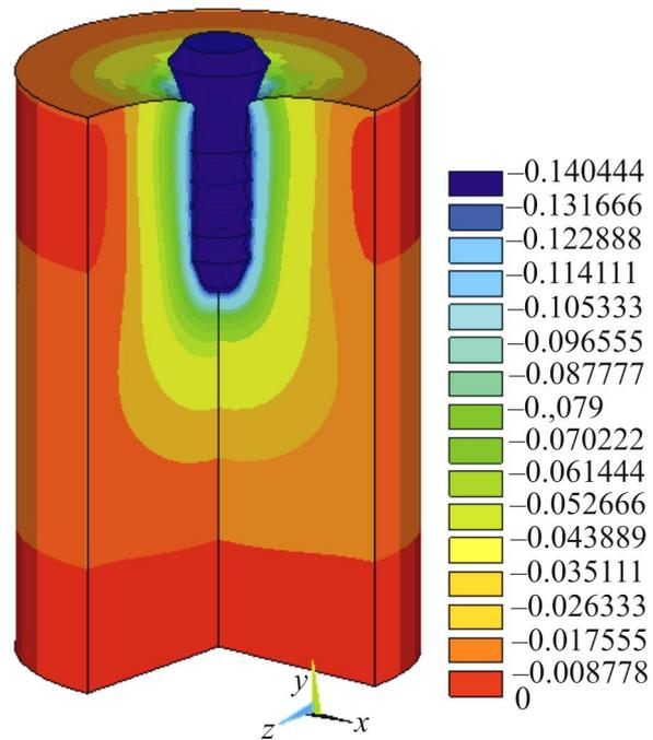
Fig. 7. Displacement along y axis: implant  $h = 13$  mm,  $d = 4$  mm,  $F=5$  N, the bottom of the sample and its lateral surface are fixed,  $\Delta Y_{\max} = 0.14$  mm
