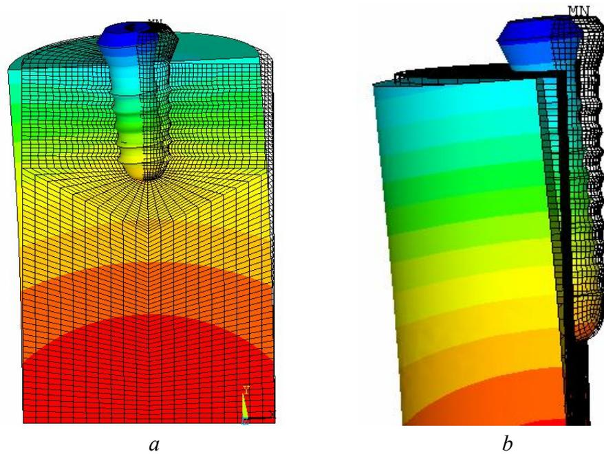
Fig. 11. Implants under influence of the pair of forces moved to the side, pulling the sample itself. Bottom is fixed (one can see how the lateral surface of the sample is curved; the transparent grid is the position of implant before the loading): *a* is longitudinal shear; *b* is lateral view of longitudinal shear
