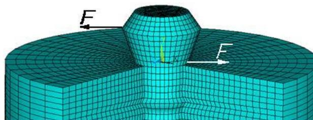
Fig. 10. A pair of forces applied to the top of the implant at different points.  $F = 1.25 \text{ N}$
