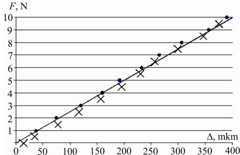
Fig. 3. Dependence of the longitudinal displacement of the implant  $\Delta$  (mkm) on the value of the compressive force  $F$  (N)
