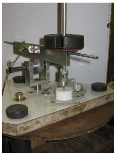
Fig. 1. Photo installation to determine the stiffness coefficients for the translational degrees of freedom
